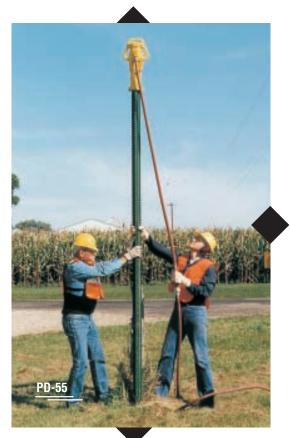
asily operated by one man, Rhino Post Drivers deliver up to 1700 blows per minute. One moving part, a reciprocating piston, strikes directly on the Post or Drive Cap. The Drivers have low air consumption rates, are light-weight and hand portable, ideal for driving in places that are hard to reach. All you need
